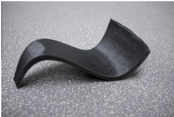
Fig. 5. Example of RepRap print quality – close-up photograph of the spoon rest.
