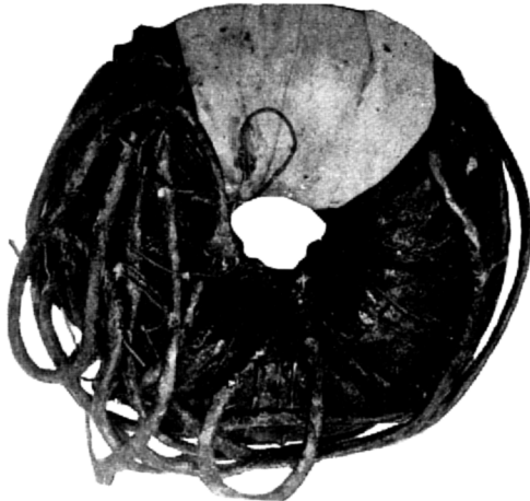
Fig. 18—Loading Coil with Winding Completed
